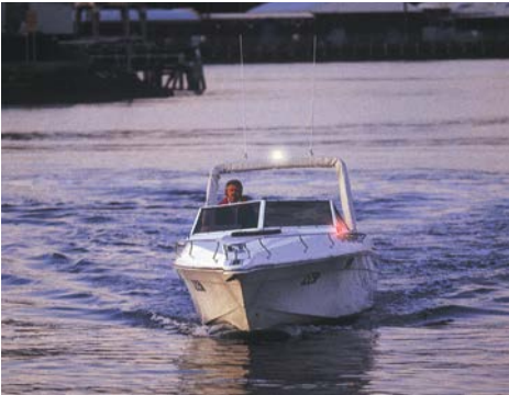
A powerboat with all round white light over the centreline, and sidelights.
